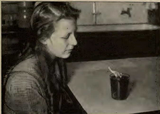
FIG. 20. The water rises through the lamp wick by capillary attraction.
